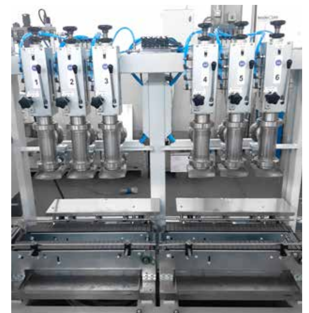
Tinting system feeder
