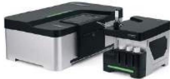
BeNano with BAT-1 titrator
